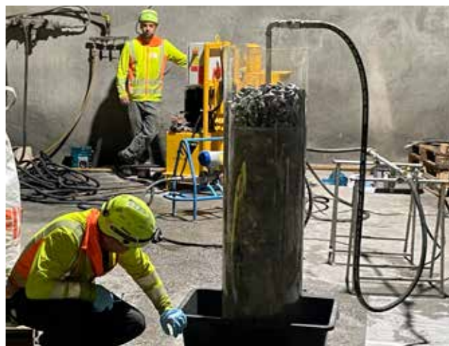
Application of the innovative hybrid injection system HIS during a presentation in the Hagerbach Test Gallery in Switzerland
