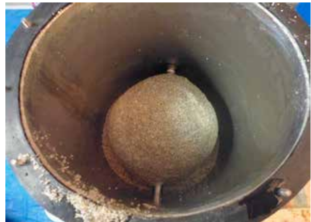
7 HIS column test according to DIN 19631 HIS-Säulenversuch nach DIN 19631
